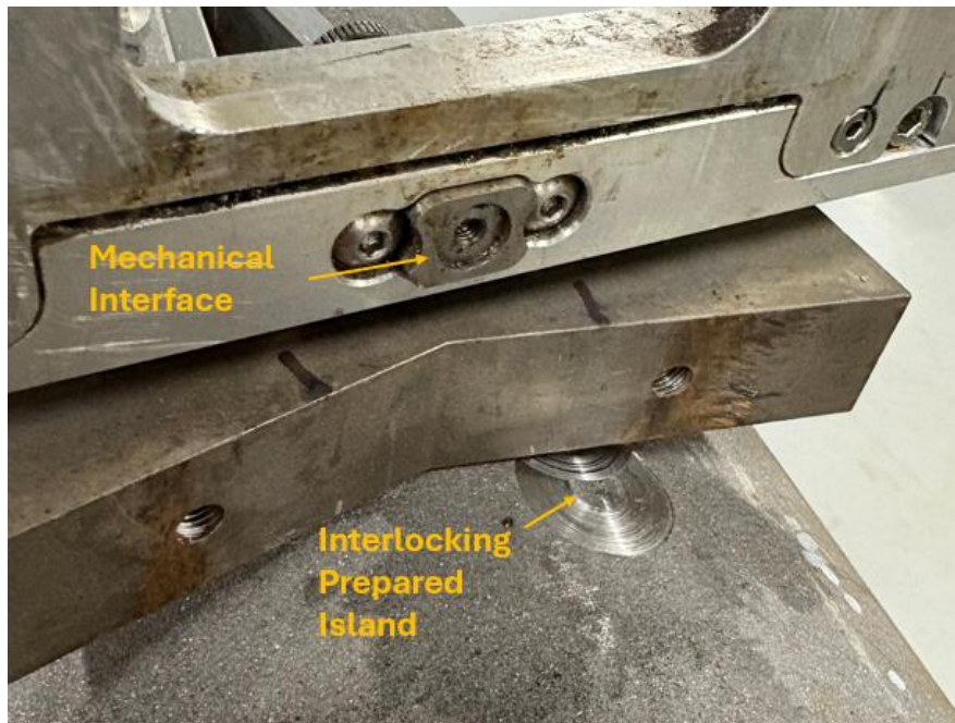
Figure 10: Mechanical Interface for Anti-Rotation
