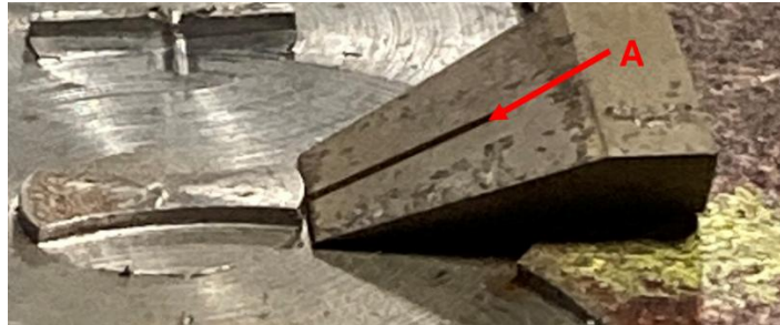
Figure 1: Blade with Labelled Stretch Passage (A)
